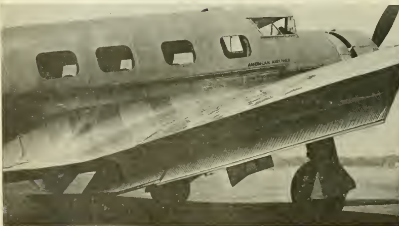
Flaps on the Vultee V-1A transport in lowered position
